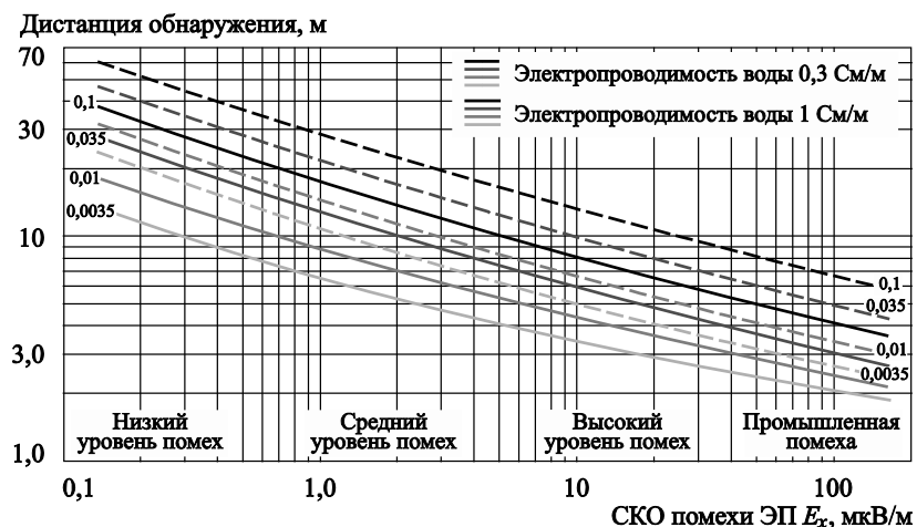
Fig. 3. Estimates of possible electric detection distances for marine objects with EDM = 0.0035–0.1 A·m: sea water conductance 0.3–1 S/m
